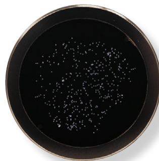
Each single star receives light from the high-power LED via a single optical fiber. Sixteen fiber-optic blocks, each for the northern and southern hemisphere are used to cover the entire star field.
