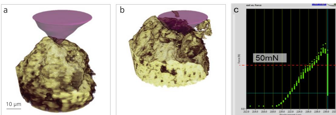
Figure 3. Nanoindentation of dentin. (a) 3D rendering of dentin sample before cracking. The indenter tip is visible above the sample. (b) 3D rendering of the same sample after the indenter tip has been driven into the sample and a piece of dentin has fractured off. (c) Force-displacement curve. The fracture event is clearly visible. Courtesy The University of Manchester.
