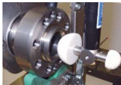
Fig. 2: Self-centering probing with active probe
