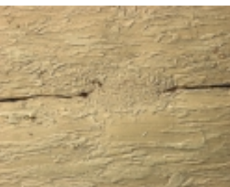
C-DIC Turbulence in the material being welded, which can only be suspected in brightfield, is clearly highlighted in C-DIC.
