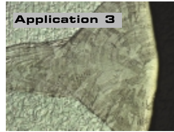
Application 3 Laser weld of a mixed joint of highly alloyed materials. The transition between the welded material and the basic material is tested. In the DIC contrasting technique, the internal structures of the welded material and the basic material are highlighted particularly well.
