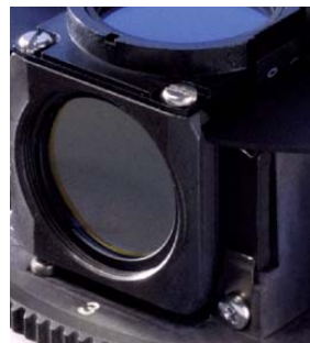
Figure 9a: C-DIC prism slider: the C-DIC prism can be rotated azimuthally using the large knurled ring; the image contrast is varied using the knurled adjusting screw (change to the phase difference \psi , see text).
