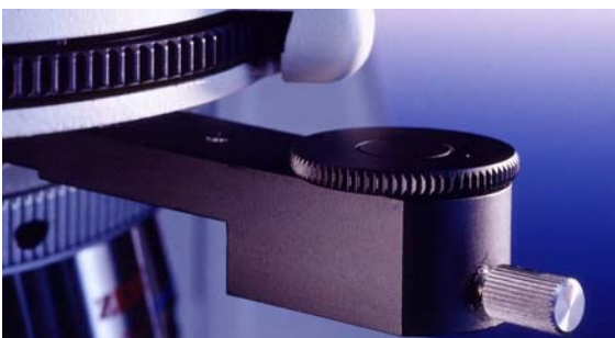
Figure 9a: C-DIC prism slider: the C-DIC prism can be rotated azimuthally using the large knurled ring; the image contrast is varied using the knurled adjusting screw (change to the phase difference \psi , see text).
