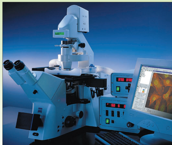
Figure 2. Axiovert 200 mot — the optimum platform for FRET investigations in living cells.
